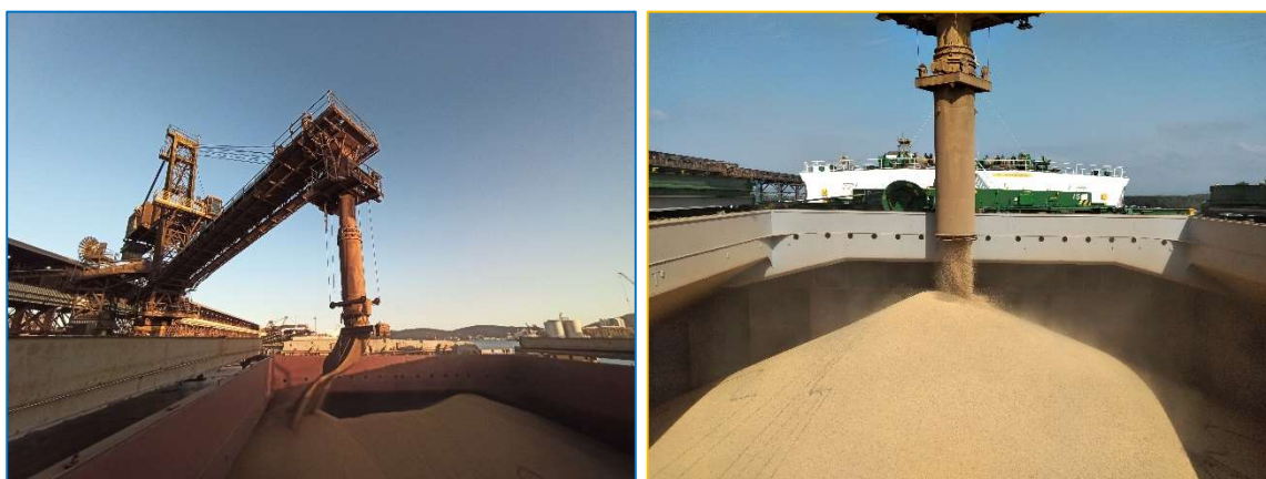
Pictures 29 & 30: Soya beans being loaded with spouts. Source: Proinde
