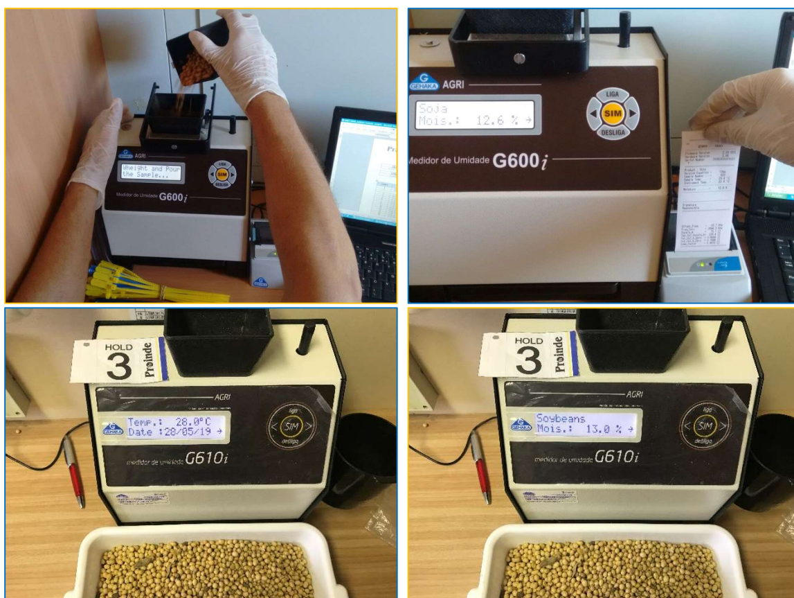
Pictures 49 to 52: Soya beans being tested for temperature and moisture content concomitantly with the loading. Source: Proinde
