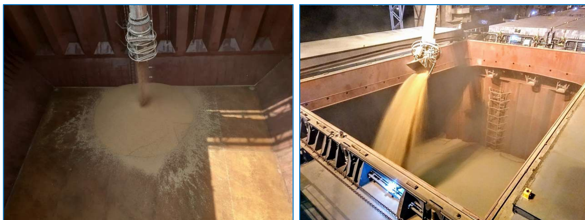
Pictures 13 & 14: soya beans being poured into the holds of bulk carriers in the early stage of loading. Source: Proinde
