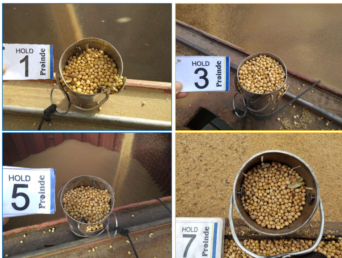
Picture 39 to 42: Soya beans samples being drawn from the hold concomitantly with the loading. Source: Proinde
