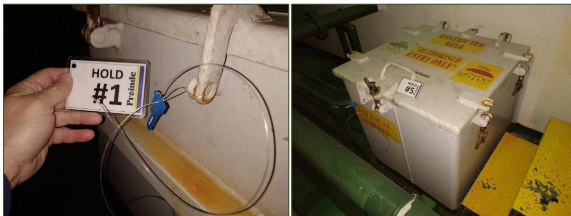
Pictures 31 & 32: Sealing of hatch covers and manholes on completion of loading. Source: Proinde
