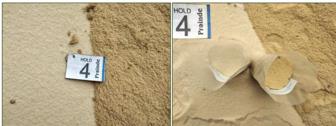
Pictures 17 & 18: Raw sugar exposed to rainwater (right part of the pictures). Source: Proinde
