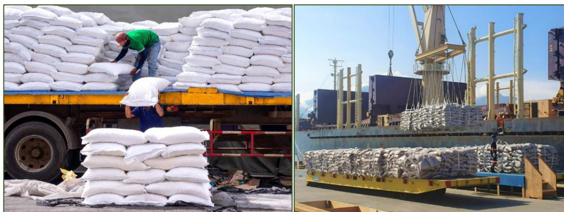
Pictures 13 & 14: Loose bags being placed on slings (left) and pre-slung bags being loaded. Source: Shutterstock/Properto
